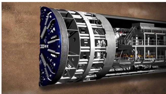
Figura 14: Tunnel Boring Machine. [23]
